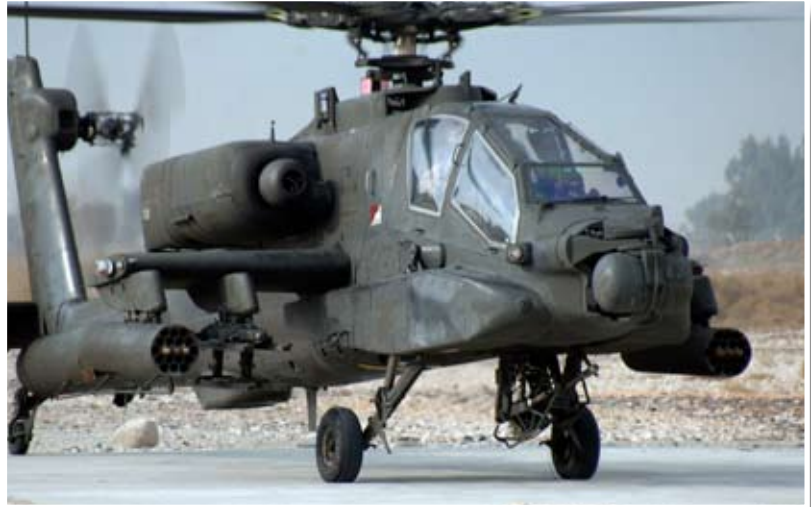
The four-blade, twin-engine AH-64 Apache attack helicopter is among the aircraft handled by the 1108th AVCRAD. U.S. Army photo
